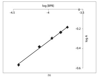
Figure 4 Limiting logarithmic plots to evaluate the stoichiometry of QTF-BPB ion-pair complex in method A: (a) variation of [QTF] and (b) variation [BPB].
