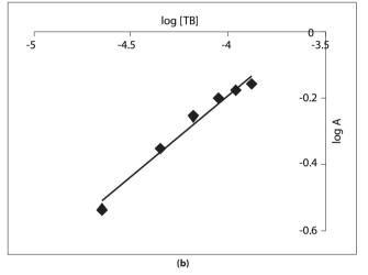
Figure 5 Limiting logarithmic plots to evaluate the stoichiometry of QTF-TB ion-pair complex in method B: (a) variation of [QTF] and (b) variation [TB].
